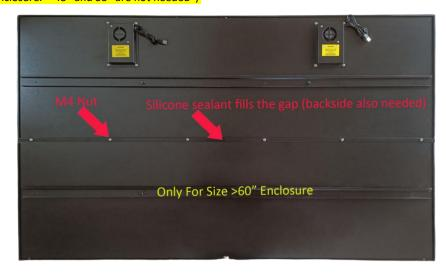
4. Assemble the front enclosure. (Components: 4 front frames, M4 flange nuts, M4 socket wrench).
