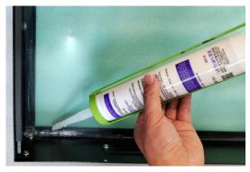
8. Finished, put the front enclosure flat on the ground and let the silicone sealant cure for about 1 hour, then remove the acrylic protective film.
