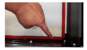
6. Remove the front side protective film of acrylic (facing human side) and install the glass/acrylic .
