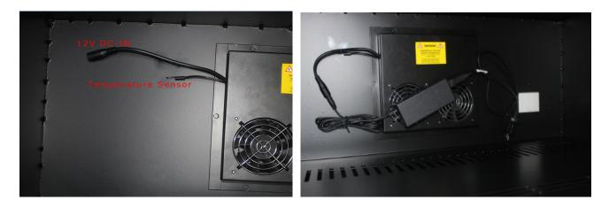
3. Pass all cables through this hole and use the screws fix the waterproof cover.
